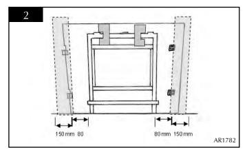
2.2 Separate the back and front sections of the frame. The frame must first be opened to 90° (right angles) to the back panel.
